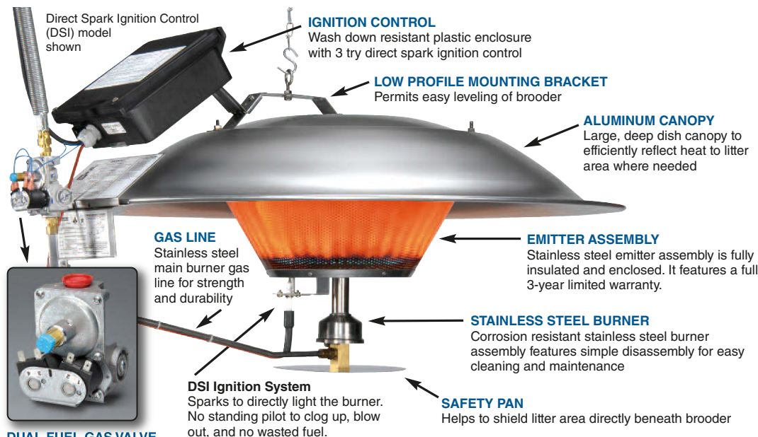
Maintenance Friendly The main burner orifice is quickly accessed by sliding back the quick release bracket shown above
